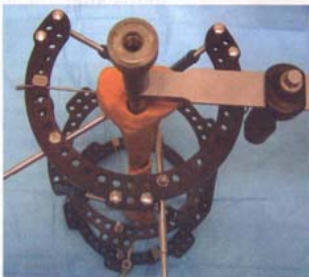
(Above) Top view of sawbone demonstration showing no contact between the rod and the external fixation pins. This is what allows insertion of the nail and avoids infection.
